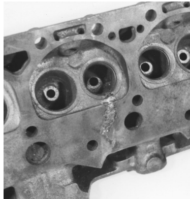
Remove Excess Plug Material
