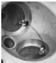
Drill Holes for Plugs
