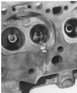
Cut Off and Peen the Plugs
