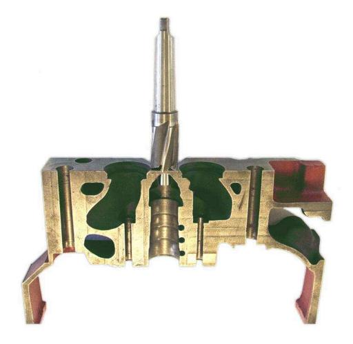
NOTE: Unless cracks extend to the valve seat area, valve seats do not need to be removed during nose plug machining and installation.
